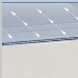
Angled one-way air discharge
