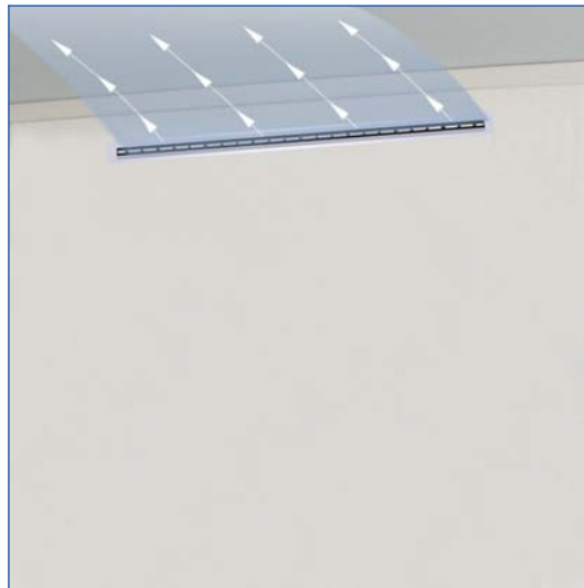
Angled one-way air discharge
