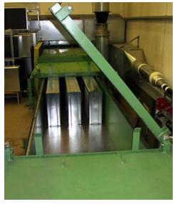
The test run, a double-walled, sound insulated and airtight stretch of channel, is attached to the reverberation chamber. The channel has a part where the channel width can be varied, which means that sound attenuator elements (splitters) of different widths and distances can be tested. Sound attenuator parameters such as insertion loss, air-regenerated noise and pressure loss
