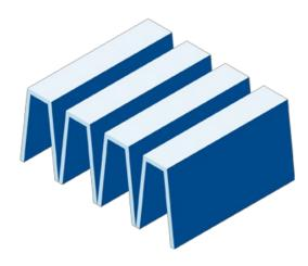
HEPA filters with filter class H13 are ideal for indoor air cleaning. They are used as standard in operating theatres or clean rooms (e.g. in micro-chip production) and reliably filter 99.95% of all virus-contaminated aerosols out of the indoor air, even at high air change rates. H14 filters achieve an efficiency of 99.995%, but also have almost twice the energy consumption of an H13 filter. Furthermore, H14 filters offer only a minimal advantage in normal, non-medical applications
